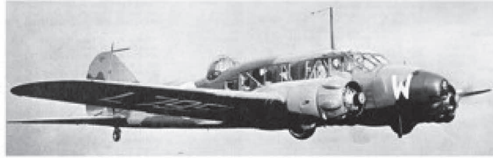
An Avro Anson fitted with Mk 1 Radar
